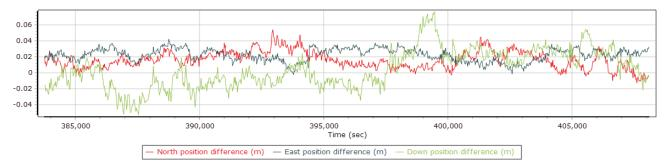
The data was collected in the Thames Estuary, where Ordnance Survey OSNet GNSS reference stations provide the data necessary to compute a SmartBase post-processed VRS network. The Applanix SmartBase (ASB) technology allows the computation of a centimetric-accurate position solution, with distances to the nearest reference station on the order of 20-60 km. A comparison was then done between the ASB solution and that from PP-RTX. The results are shown above.
