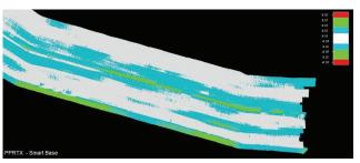
Differencing the two surfaces confirms the level of agreement, with no differences greater than 10 cm, and the majority less than 5 cm.
