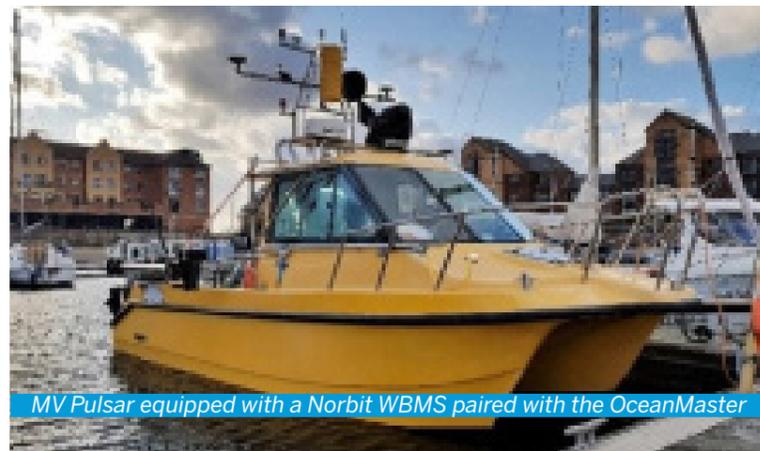
MV Pulsar equipped with a Norbit WBMS paired with the OceanMaster
