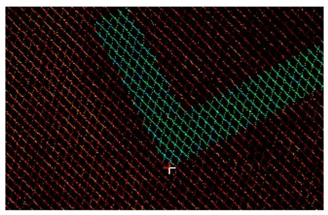
Figure 7: GCP Point Measurement in Trimble Business Center
