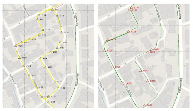
Figure 4: Left - Vertical GCPs, Right - 3D GCPs for horizontal performance
