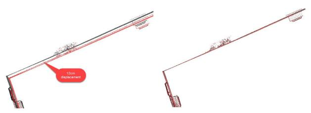
Figure 9: Horizontal Displacement both before and after LiDAR QC
