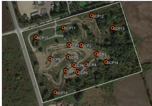
Figure 4: Applanix Test Field Showing GCP Layout
