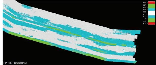
Differencing the two surfaces confirms the level of agreement, with no differences greater than 10 cm, and the majority less than 5 cm.
