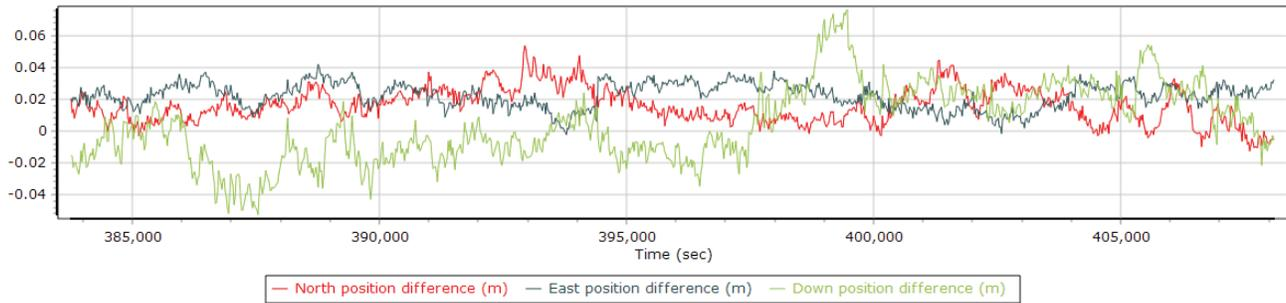
The data was collected in the Thames Estuary, where Ordnance Survey OSNet GNSS reference stations provide the data necessary to compute a SmartBase post-processed VRS network. The Applanix SmartBase (ASB) technology allows the computation of a centimetric-accurate position solution, with distances to the nearest reference station on the order of 20-60 km. A comparison was then done between the ASB solution and that from PP-RTX. The results are shown above.
