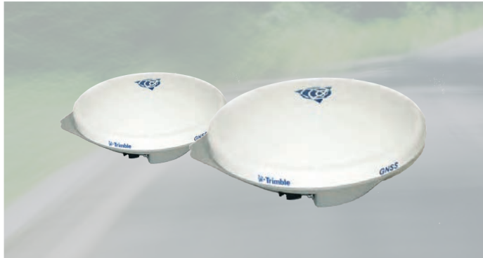
GAMS GAMS (GNSS Azimuth Measurement Subsystem) integrates an IMU with a 2-antenna heading measurement system. By utilizing a carrier phase differential GNSS algorithm to measure the relative position vector between the two antennas, GAMS continuously calibrates the IMU and ensures that azimuth does not drift (as long as there is GNSS coverage).
