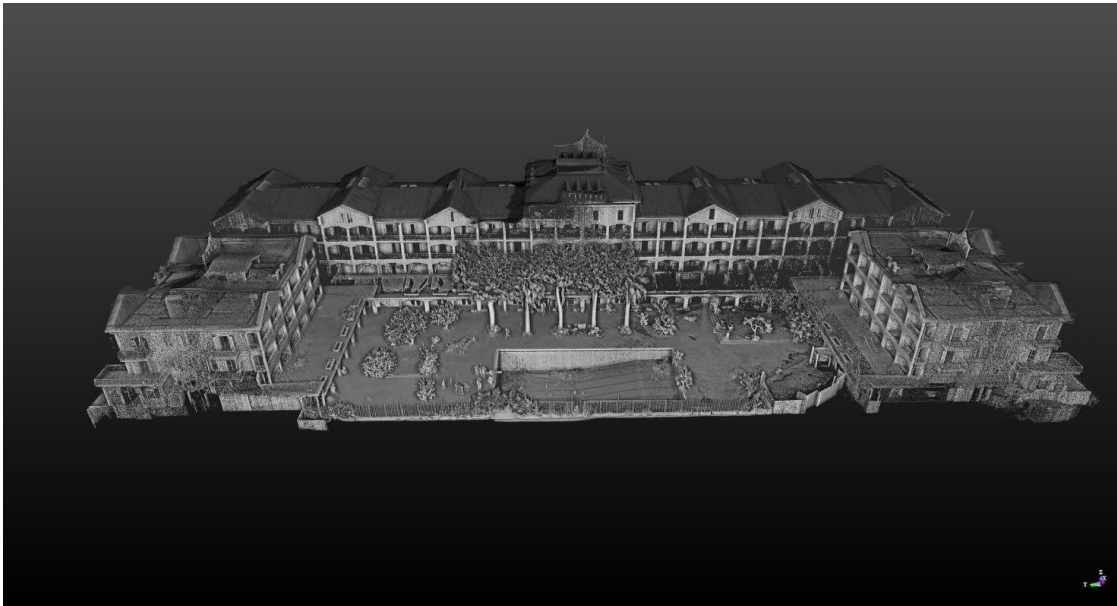
TIMMS & UAV point clouds (roofs) based on reflectance
