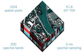
Hperspectral cube and top level specs for Mjolnir-1024
